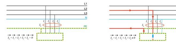
Residual currents are composed of a capacitive part and a resistive part.
